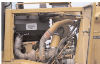
DCL's Mine-X Sootfilter diesel particulate filter system installed on a Caterpillar D8T dozer.
