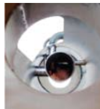
The inside of Huss' online burner. The burner keeps exhaust temperatures above 300°C even at low load conditions.
